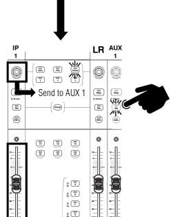
In Sends on Rotaries mode, Strip Rotaries are used to control send levels to the active mix, with the channel faders remaining as level controls to the Main Mix.
