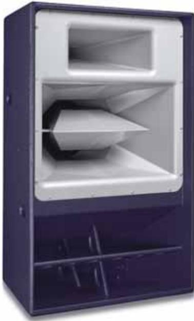
Evo 6E is a high intensity, three way loudspeaker. It combines a Funktion-One signature 10" midrange with a horn loaded 15" mid-bass and a 1.4" compression driver in a compact cabinet. This results in class leading efficiency and performance. The Evo 6E is also available with passive high frequency crossover, giving the option of two way amplification.
