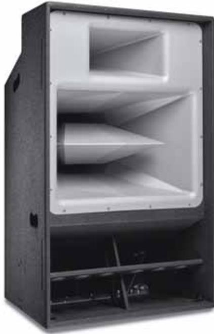
Evo 7T is a very high intensity touring loudspeaker, which features a 10" Funktion-One signature midrange with a horn loaded 15" mid-bass and a 1.4" compression driver. It has 35° of horizontal dispersion and physically arrays at 30°. A three wide array gives smooth coverage to 100°.
