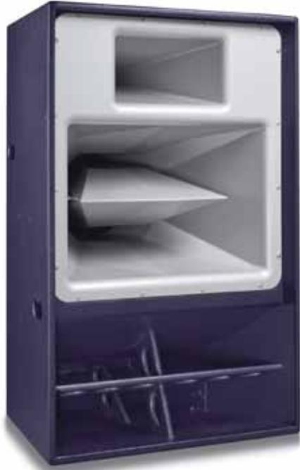
Evo 7E is a very high intensity, three way loudspeaker. It combines a Funktion-One signature 10" midrange with a horn loaded 15" mid-bass and a 1.4" compression driver in a compact cabinet. This results in class leading efficiency and performance. The Evo 7E is also available with a passive high frequency crossover, giving the option of two way amplification.
